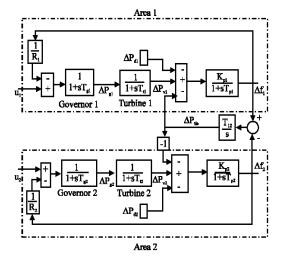
Fig 5.2 Complete block diagram of two- area LFC
